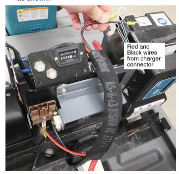
5. Connect the red cable to the (+) terminal on main contactor and the black cable to the negative stand-off.
