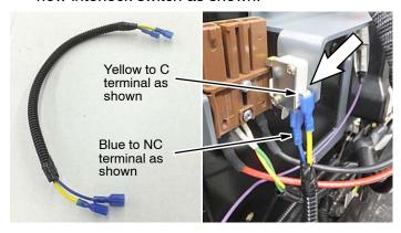
7. Connect the other end of extension wire harness to the blue and yellow wires that were originally connected to the old interlock switch.
