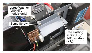
4. Route the red and black wires from the new charger connector through the protective sleeve as shown.
