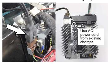
3. Turn key on to confirm the charger interlock switch disables the machine during the charge cycle. An audio alarm (horn) will beep nine times repeatedly indicating that the charger is plugged into machine which also disables the machine. If the alarm fails to beep, check the interlock switch for proper installation. Check wire connections and roller alignment. Repeat step.
