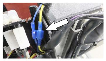
8. Secure the extension wire harness and the seat wire harness to panel with cable-tie as shown.
