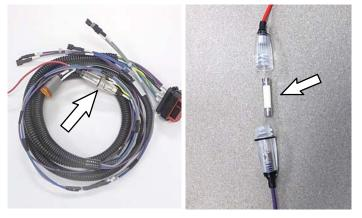
10. Connect the new telemetry harness to the following components. Secure harness with cable-ties.
