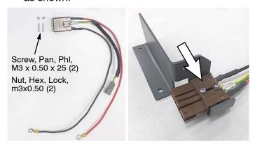
Connect the new interlock switch to bracket with hardware as shown.
